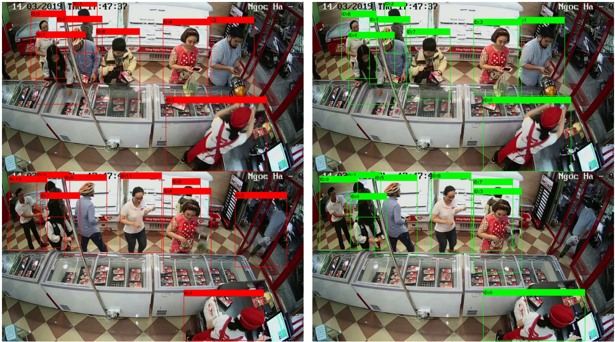
Fig. 7. Qualitative comparison result on two methods. Red bounding boxes are DeepSORT’s visualization and green bounding boxes are the visualization of our method. Our method performs tracking better than DeepSORT after a complete occlusion. The 9th ID changes to the 11th ID, compares with the 8th ID, whose prediction is more stable. Best viewed on color display.
